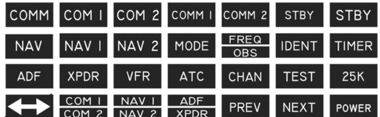
GoFlight's MagLabels are used to label the displays and buttons on the GF-166 for easy reference during flight. Using a pair of scissors, carefully cut out the labels that you wish to place on the panel to correspond with functions you have assigned using GFConfig.
