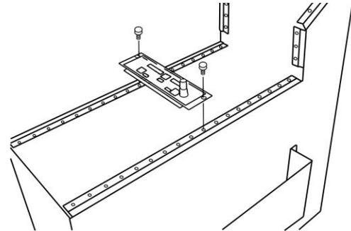
Installing the GF-166 into the GoFlight Flight Deck Console.
