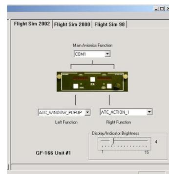
The Main Avionics Function list contains entries for all radio types including COM1, NAV1, COM2, NAV2, ADF and Transponder. When you select one of these function types, the behavior of the rotary knobs, dual displays, and center function button are configured to operate as the type of radio you have selected. The Left and Right Function buttons are unaffected by the Main Avionics Function selection.
