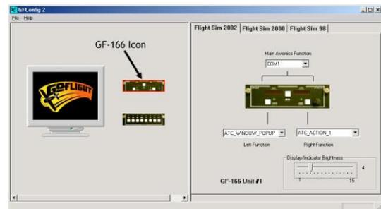
Selecting the GF-166 device icon in the Device View.
